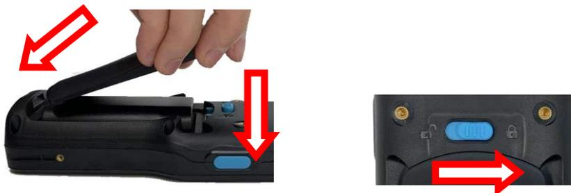
■ Remove the battery cover and the battery
