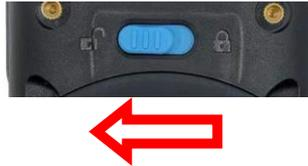
2. Grab the battery cover from the two recesses and gently lift upward, stop when you feel a resistive force. Press the battery cover against the battery, and lift the battery upwards until you remove the battery. (The process follows the principle of lever).
