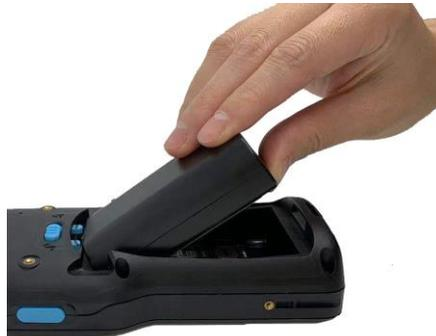
2. Make sure the battery release latch is in the unlocked position.
