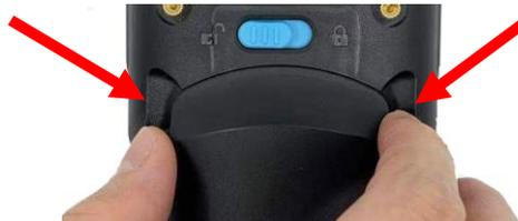
3. There are two ways to remove the battery. First one is by pulling the pull tab in the battery compartment to remove the battery. Make sure the pull tab stays inside of the battery compartment when closing the cover.
