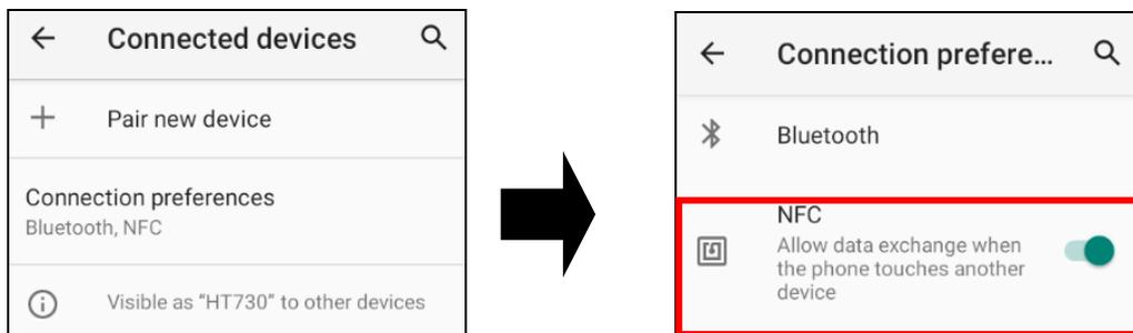
3. Make sure that both devices are unlocked and have NFC turned on. Also make sure that the NFC antenna area of HT730 and the other devices' NFC area are close to one another. Slightly moving the phones until a connection is made. Tap the screen.
