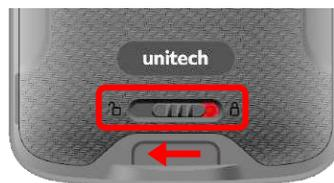
2. Lift the battery cover up to 45 degrees (45°) angle by pulling the bottom-left corner up then gently take the cover off.
