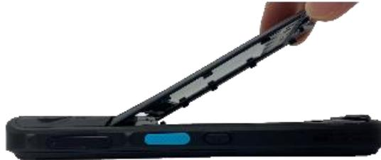
3. Align the battery cover with the recesses of the battery compartment and press the battery cover down to secure in place. Make sure there is no gap between the device and the battery cover.
