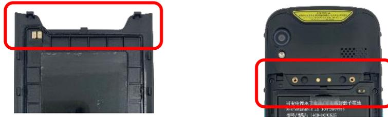
2. Insert the battery cover up to 45 degrees (45°) angle, from top to bottom.
