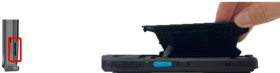
3. Align the battery with the bottom slot in the battery compartment.
