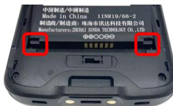
4. Press down the battery and secure in place.
