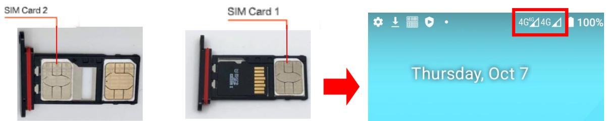
**(A)** Put in two SIM Cards **or (B)** Put in one SIM Card and an SD Card.
